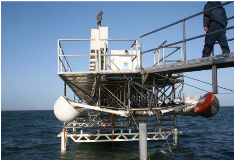
Figure 4-7: The Wave Star deployed at the Wave Danish Test Station, Nissum Bredning [56]
